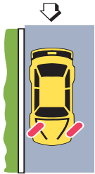
When the front of a parked vehicle points downhill, wheels should be turned toward the curb or shoulder of the road.
